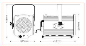
Compact, lightweight and powerful 2/2.5KW fresnel spotlight. It features an extremely wide beam angle and includes a height adjustable, robust G22 lamp-base, screw focus, strong tilt lock and double-microswitch interlock for safe lamp replacement. A colour frame, safety guard and 1.5m mains cable are included as standard.
