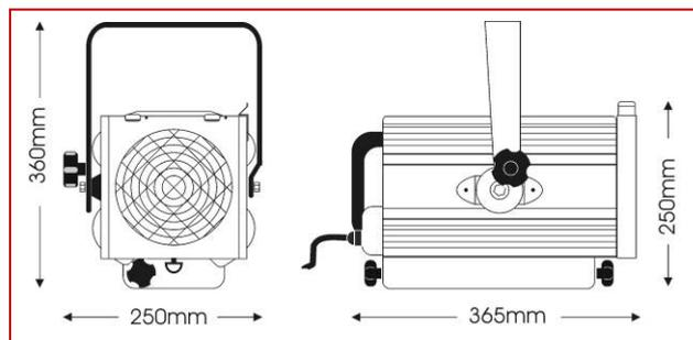
Quality 1/1200W fresnel spotlight including screw focus variable spread soft-edged beam, front hinging lamp tray, tilt lock and double-microswitch interlock for safe lamp replacement.
